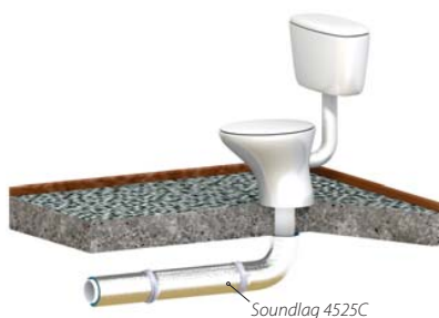
BCA Section F5.6 Compliant Non-habitable room
